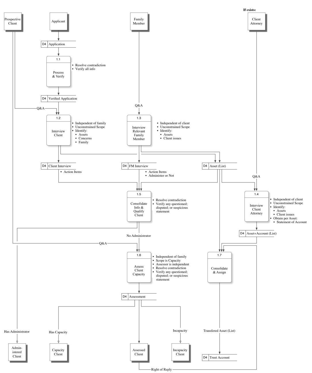
This is presented in SSADM notation (often called Data Flow Diagrams), such that the processes and their interaction can be analysed.
